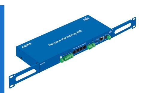
Perseus Monitoring 150 connects external physical sensors (°C, %RH, A, V, ...), DI (Digital Inputs), WLD (Water Leak Detection) zone, DO (Digital Outputs) and 3<sup>rd</sup> party meters via LAN or RS-485 (Modbus/RTU).
